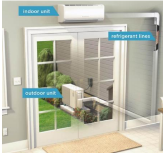
Electric heat pump
