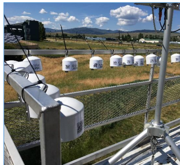
Collocation of PurpleAir sensors with reference monitors at the USFS Missoula Fire Science Lab
