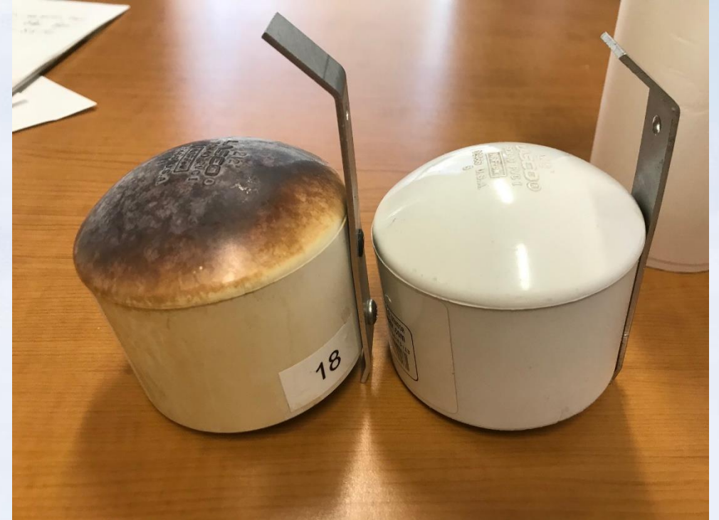
A P-TAQs PurpleAir unit that has been exposed to the Phoenix sun for over a year.
