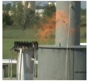
Flare **DRE 99.2%** at steam-to-vent gas (SVG) ratio of 0.29.
