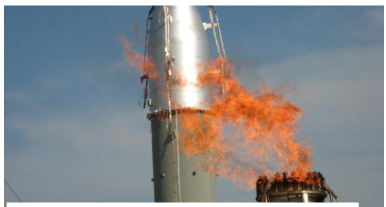
High DRE. The dark orange flame and lack of visible steam are excellent visual indicators of the flare being operated at high DRE.
