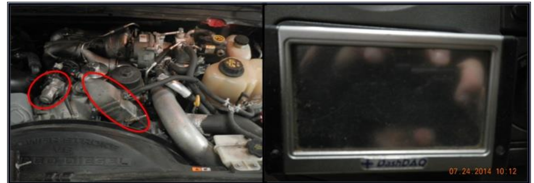
EGR electronic disablement (all EGR parts present and sensors plugged in)
